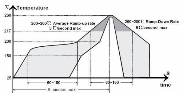
Peak temperature.  $260^{\circ}\text{C} \pm 5^{\circ}\text{C}$  (10sec. max.) Reflow is permitted 2 times
