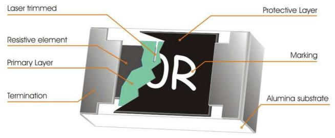
Fig 1. Construction of Chip-R
