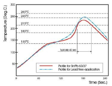
Fig 3. Infrared soldering profile for Chip Resistors
