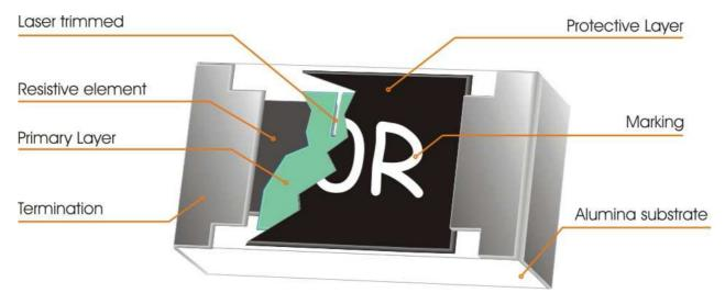
Fig 1. Construction of Chip-R
