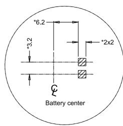
Position & size of soldering pads (For customer reference only)
