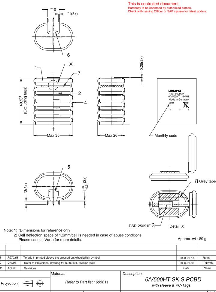
Dimensions in mm Prepared & Checked Verified & Approved 695811 401 Dwg. No: TitisWS Tolerance: As specified 2006-55750 306 012 09-06 VKB Order No: Scale: Rights reserved to make technical changes, as a result of further development, without notice. This drawing is the property of VARTA Microbattery **□VART** and must not be copied or disclosed to a third party without the written consent of VARTA Microbattery.
