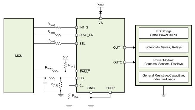
Figure 38. Typical Application Diagram
