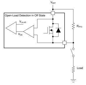
Figure 31. Open-Load Detection in Off-State
