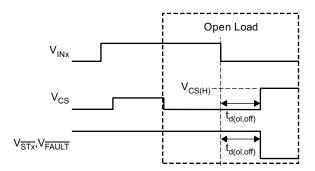
Figure 3. Open-Load Blanking-Time Characteristics
