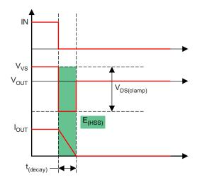
Figure 27. Inductive Load Switching-Off Diagram
