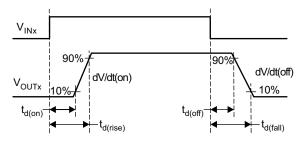
Figure 1. Output Delay Characteristics
