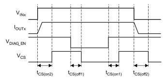
Figure 2. CS Delay Characteristics
