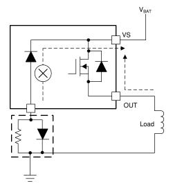
Figure 35. Reverse-Current External Protection, Method 2
