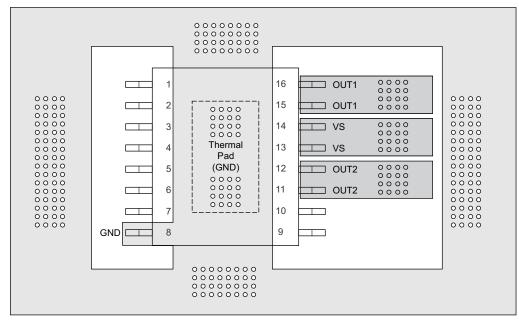
Figure 44. Layout Example Without a GND Network
