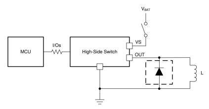
Figure 33. Protection for Loss of Power Supply
