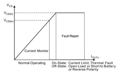
Figure 24. Current-Sense Output-Voltage Curve
