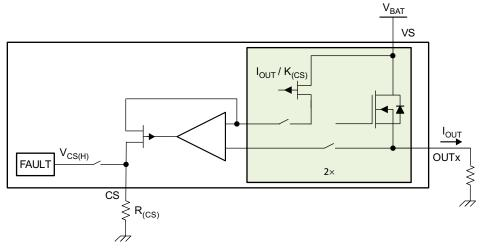
Figure 23. Current-Sense Block Diagram
