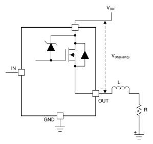
Figure 26. Drain-to-Source Clamping Structure
