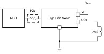
Figure 36. MCU I/O External Protection
