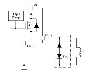
Figure 30. Protection With External Circuitry
