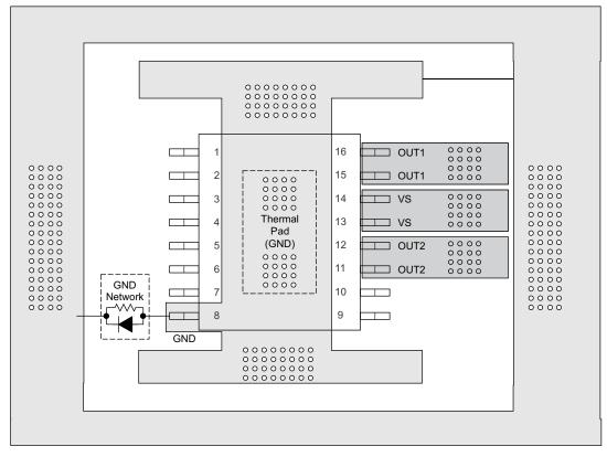
Figure 45. Layout Example With a GND Network
