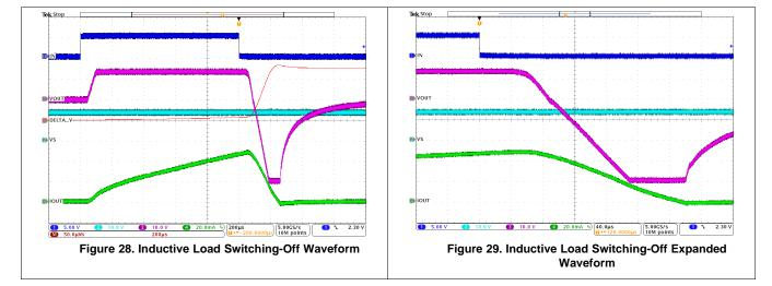
Note that for PWM-controlled inductive loads, it is recommended to add the external freewheeling circuitry shown in Figure 30 to protect the device from repetitive power stressing. TVS is used to achieve the fast decay. See Figure 30 for more details.
