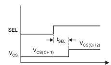
Figure 4. Multi-Sense Transition Delay
