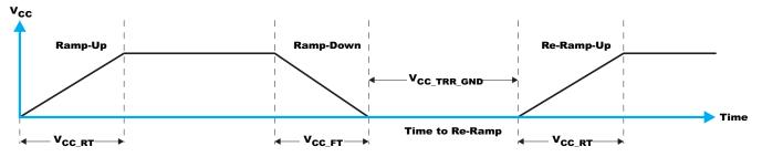
Figure 39. V<sub>CC</sub> is Lowered Below 0.2 V or 0 V and Then Ramped Up to V<sub>CC</sub>
