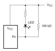
Figure 35. High-Value Resistor in Parallel With LED
