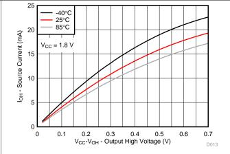
Figure 11. I/O Source Current vs Output High Voltage for Different Temperature ( $T_A$ ) for  $V_{CC}$  = 1.65 V
