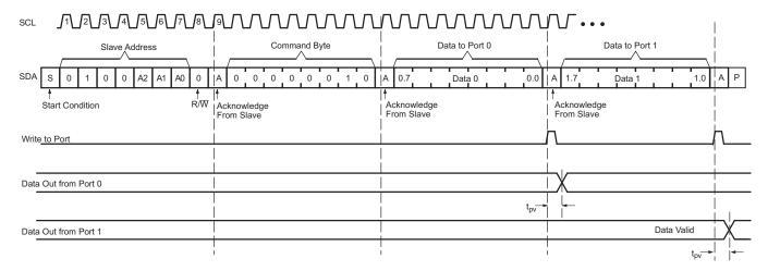
Figure 28. Write to Output Port Registers
