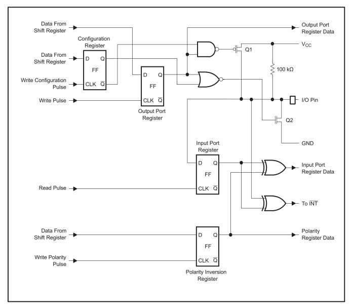
Figure 23. Simplified Schematic of P-Port I/Os
