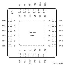
The exposed thermal pad, if used, must be connected as a secondary ground or left electrically open.
