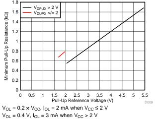
Figure 38. Minimum Pull-Up Resistance ( $R_{p(min)}$ ) vs Pull-up Reference Voltage ( $V_{CC}$ )
