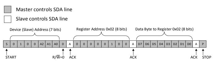
Figure 27. Write to the Polarity Inversion Register
