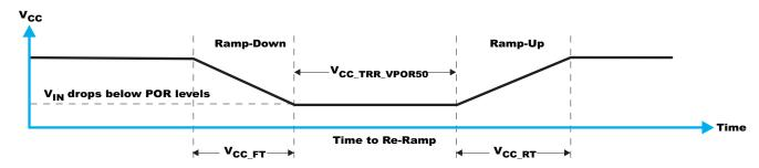
Figure 40. V<sub>CC</sub> is Lowered Below the POR Threshold, Then Ramped Back Up to V<sub>CC</sub>
