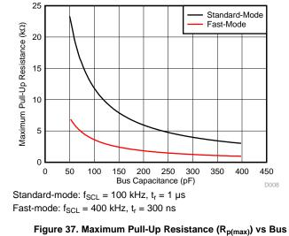
Figure 37. Maximum Pull-Up Resistance (R<sub>p(max)</sub>) vs Bus Capacitance (C<sub>b</sub>)
