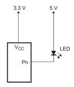
Figure 36. Device Supplied by Lower Voltage
