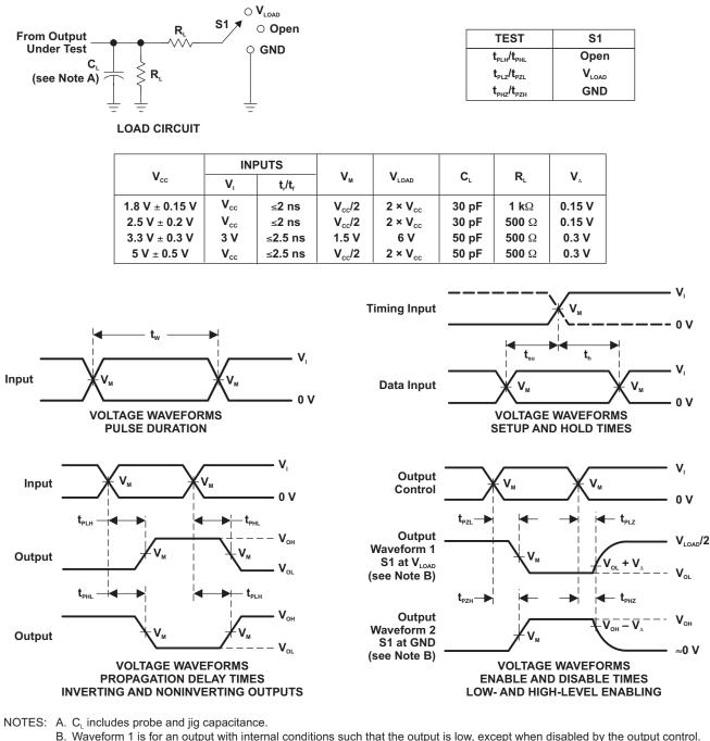
B. Waveform 1 is for an output with internal conditions such that the output is low, except when disabled by the output control.
