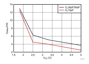
Figure 7. Enable Time vs V<sub>CC</sub>
