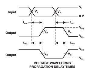
INVERTING AND NONINVERTING OUTPUTS
