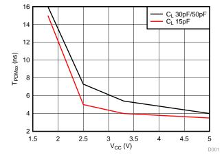
Figure 1. Propagation delay vs V<sub>CC</sub>
