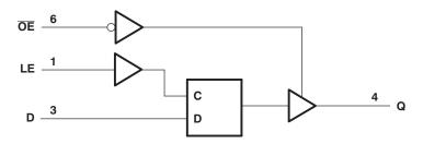
Figure 4. Logic Diagram (Positive Logic)
