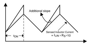
Figure 20. Slope Compensation
