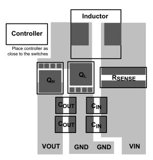
Figure 49. Power Path Layout
