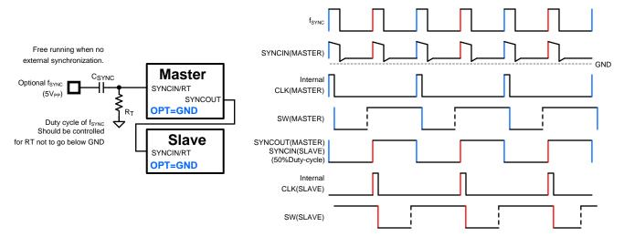
Figure 32. Dual Phase Configuration and Timing Diagram
