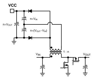
Figure 18. External Bias Supply using Transformer
