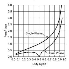
Figure 30. Normalized Output Capacitor RMS Ripple Current
