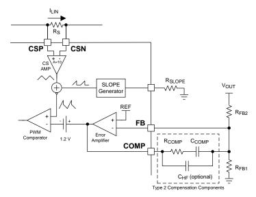
Figure 21. Feedback Configuration and PWM Comparator
