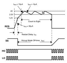
Figure 26. Hiccup Mode Overload Protection
