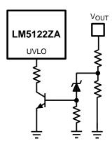
Figure 36. Output Overvoltage Protection
