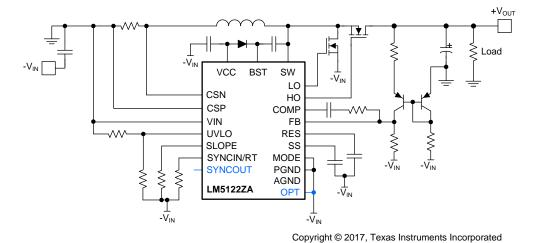
Figure 39. Negative to Positive Converter Simplified Schematic
