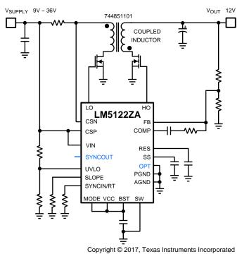
Figure 38. Non-Isolated Synchronous Flyback Converter Simplified Schematic
