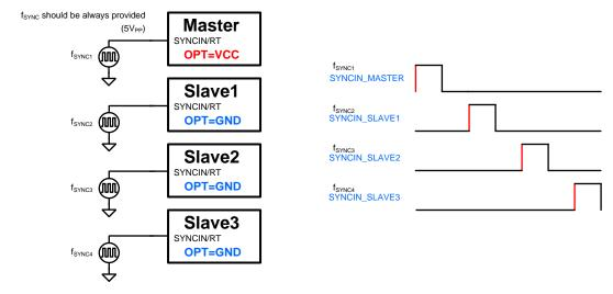
Figure 33. 4-Phase Timing Diagram Individual Clock
