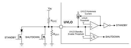
Figure 16. UVLO Remote Standby and Shutdown Control
