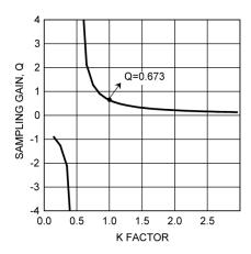
Figure 29. Sampling Gain Q vs K Factor
