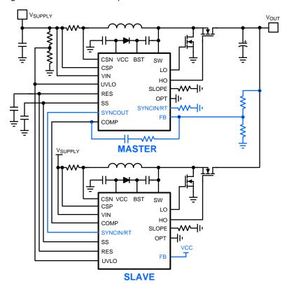
Figure 31. Dual Phase Interleaved Boost Configuration
