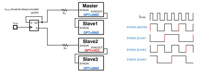
Figure 34. 4-Phase Timing Diagram Daisy Chain
