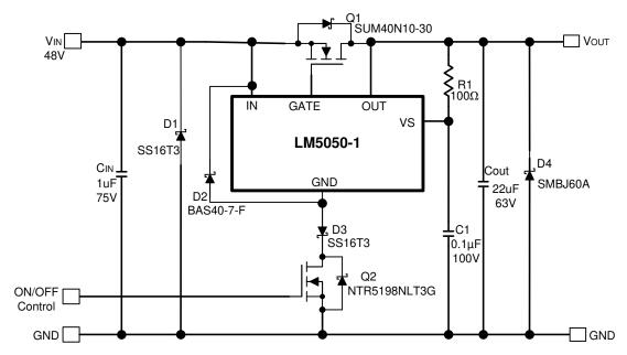
Figure 29. Reverse Input Voltage Protection With IQ Reduction Schematic
