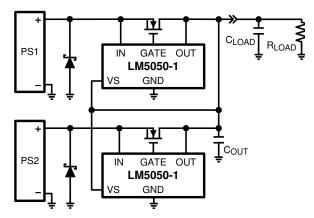
Figure 28. ORing of Two Power Sources
