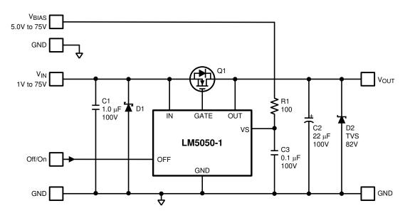
Figure 27. Using a Separate vs Supply for Low Vin Operation Schematic
