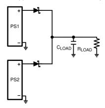
Figure 21. OR-ing with Diodes
