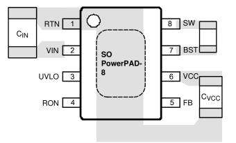
Figure 10-1. Placement of Bypass Capacitors
