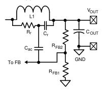
Figure 8-8. Type III Ripple Circuit
