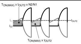
Figure 8-6. Current Waveforms for C<sub>OUT1</sub> Ripple Calculation
