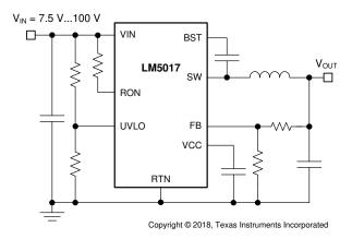
**Typical Synchronous Buck Application Circuit**
