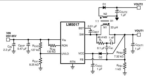
Figure 8-5. Typical Isolated Application Schematic
