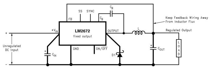
Heavy Lines Must Be Kept Short And Use Ground Plane Construction For Best Results
