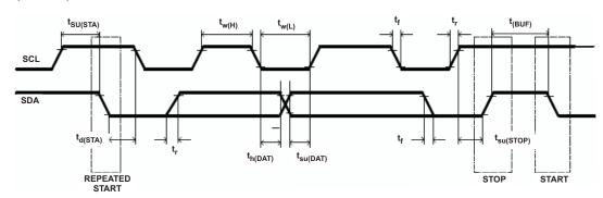
Figure 1. I<sup>2</sup>C-Compatible Interface Timing Diagrams
