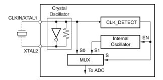
Figure 8-4. Equivalent Circuitry of the Clock Source
