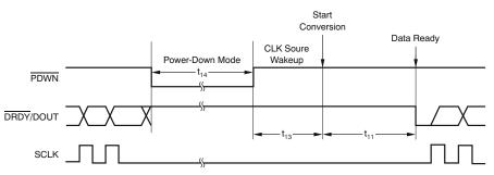
Figure 8-14. Wake-Up Timing From Power-Down Mode
