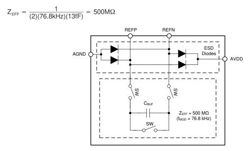
Figure 8-3. Simplified Reference Input Circuitry
