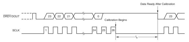
Figure 8-11. Offset-Calibration Timing
