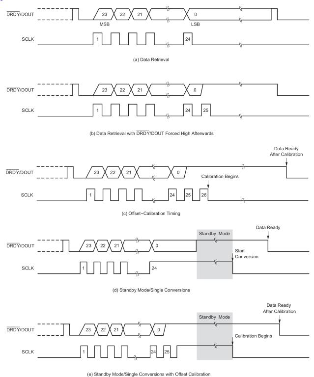
Figure 8-16. Summary of Serial Interface Waveforms
