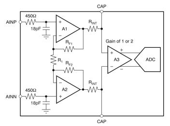
Figure 8-2. Simplified Diagram of the PGA
