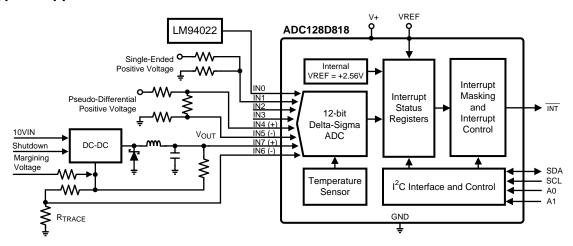
Figure 36. Hardware Monitor Application
