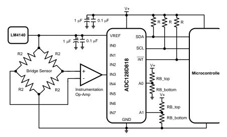
Figure 41. Bridge Sensor Application
