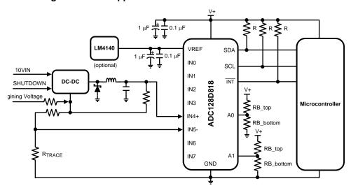
Figure 39. Power Supply Application
