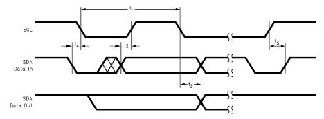
Figure 1. Serial Bus Timing Diagram
