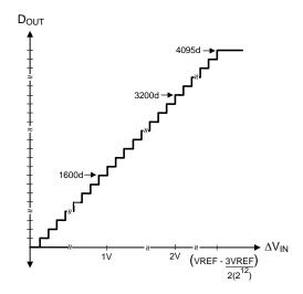
Figure 32.  $D_{OUT}$  vs  $\Delta$ VIN for a 12-Bit ADC Assuming VREF = 2.56 V.
