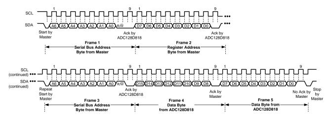
Figure 31. Serial Bus Interface Read Example 4 - Double Byte Read With Internal Address Set Using a Repeat Start
