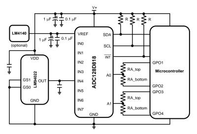
Figure 40. Temperature Sensor Applications
