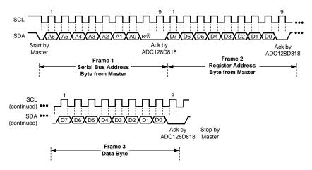
Figure 27. Serial Bus Interface Write Example 2 - Internal Address Register Set With Data Byte Write
