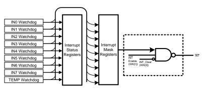
Figure 34. Interrupt Structure
