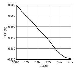
Figure 37. Total Unadjusted Error
