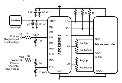
Figure 38. Typical Analog Input Application
