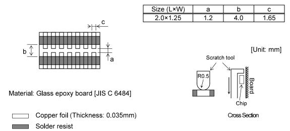
Remarks: Uniform soldering shall be conducted with solder (H60A or H63A in JIS Z 3282) by using soldering iron or soldering oven.
