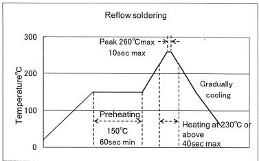
\*Ceramic chip component should be preheated sufficiently to maintain the temperature difference between the component surface and solder at 130°C or below.
