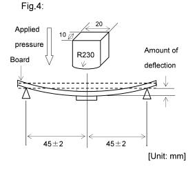
Apply pressure at the rate of 0.5mm/sec. until amount of deflection reaches 1.0mm.
