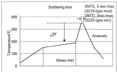
\* $\triangle$ T $\leq$ 150°C(3216-type max), $\triangle$ T $\leq$ 130°C(3225-type min)
