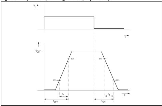
Figure 3. Input to output timings and output pulse shape
