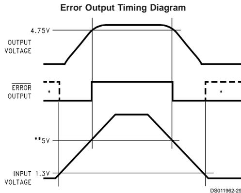
\*In shutdown mode,  $\overline{\text{ERROR}}$  will go high if it has been pulled up to an external supply. To avoid this invalid response, pull-up to regulator output.
