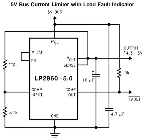
\*Output voltage equals  $+V_{IN}$  minus dropout voltage, which varies with output current. Current limits at a maximum of 1000 mA (typical).
