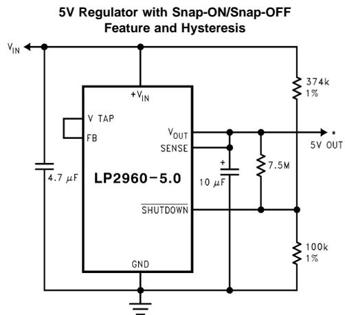
\*Turns ON at  $V_{IN} = 5.87V$
