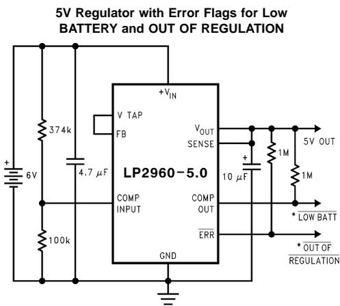
\*Connect to Logic or  $\mu P$  control inputs.
