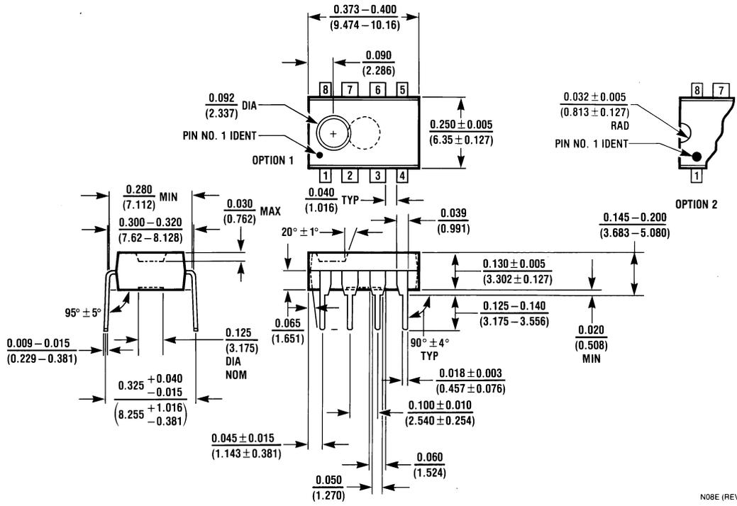
**8-Pin Molded Dual-In-Line Package**
