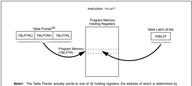
Note1: The Table Pointer actually points to one of 32 holding registers, the address of which is determined by TBLPTRL<4:0>. The process for physically writing data to the program memory array is discussed in Section 6.5 "Writing to Flash Program Memory".
