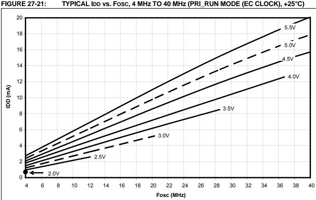
TYPICAL IDD vs. Fosc, 4 MHz TO 40 MHz (PRI\_RUN MODE (EC CLOCK), +25°C)
