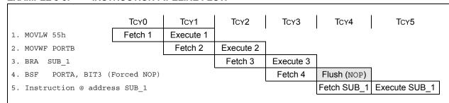
All instructions are single cycle, except for any program branches. These take two cycles since the fetch instruction is "flushed" from the pipeline while the new instruction is being fetched and then executed.
