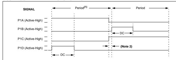
Note 1: The direction bit in the CCP1 Control register (CCP1CON<7>) is written any time during the PWM cycle.
