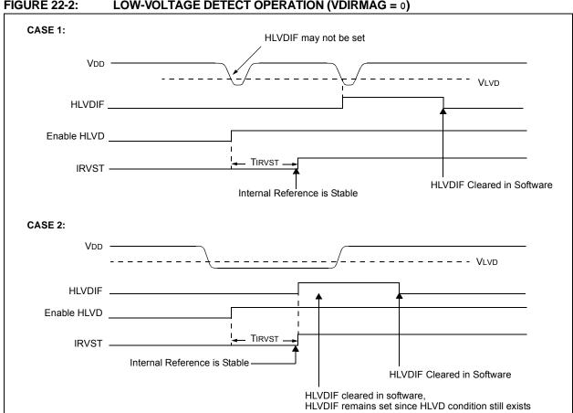
**FIGURE 22-2: LOW-VOLTAGE DETECT OPERATION (VDIRMAG = 0)**
