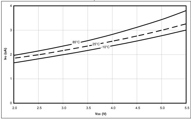
FIGURE 27-6: TYPICAL T1OSC DELTA CURRENT vs. VDD ACROSS TEMP. (DEVICE IN SLEEP, T1OSC IN HIGH-POWER MODE)
