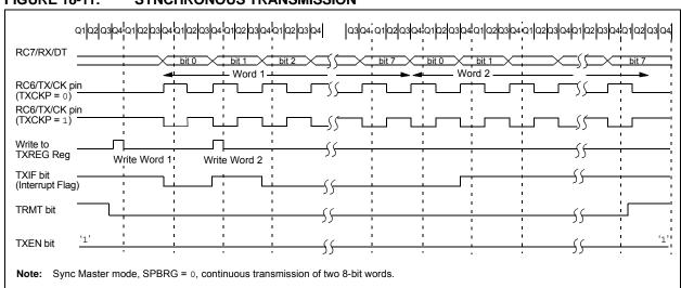
FIGURE 18-12: SYNCHRONOUS TRANSMISSION (THROUGH TXEN)
