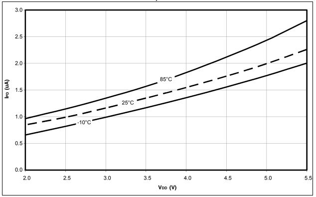
FIGURE 27-5: MAXIMUM T1OSC DELTA CURRENT vs. VDD ACROSS TEMP. (DEVICE IN SLEEP, TIOSC IN LOW-POWER MODE)
