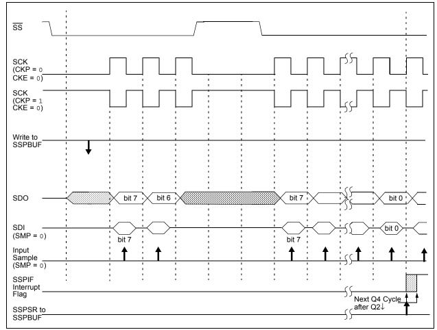
FIGURE 17-5: SPI MODE WAVEFORM (SLAVE MODE WITH CKE = 0)
