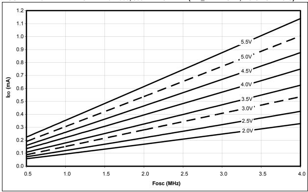
FIGURE 27-27: TYPICAL IDD vs. Fosc, 4 MHz TO 40 MHz (PRI\_IDLE MODE, +25°C)
