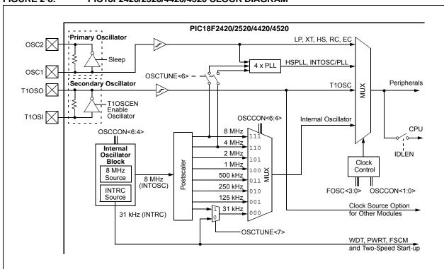
FIGURE 2-8: PIC18F2420/2520/4420/4520 CLOCK DIAGRAM
