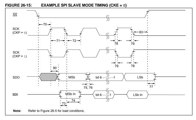
TABLE 26-16: EXAMPLE SPI MODE REQUIREMENTS (SLAVE MODE TIMING, CKE = 0)
