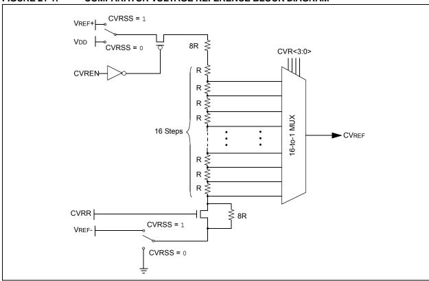
FIGURE 21-1: COMPARATOR VOLTAGE REFERENCE BLOCK DIAGRAM
