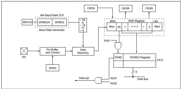
FIGURE 18-7: ASYNCHRONOUS RECEPTION
