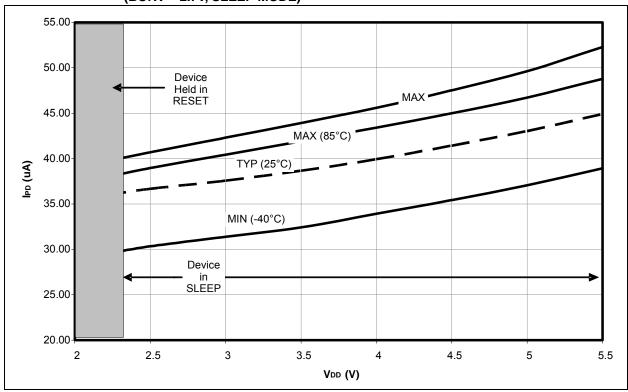
FIGURE 27-9: TYPICAL WDT CURRENT vs. VDD ACROSS TEMPERATURE (WDT DELTA CURRENT IN SLEEP MODE)
