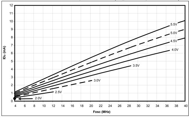
FIGURE 27-29: TYPICAL IDD vs. Fosc, HS/PLL (PRI\_IDLE MODE, +25°C)
