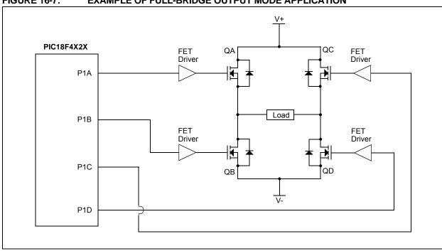
FIGURE 16-7: EXAMPLE OF FULL-BRIDGE OUTPUT MODE APPLICATION
