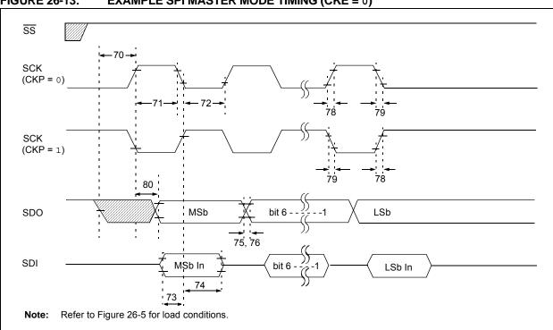
FIGURE 26-13: EXAMPLE SPI MASTER MODE TIMING (CKE = 0)
