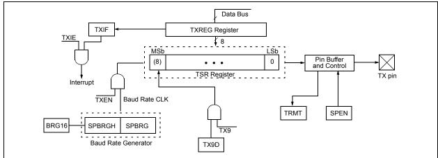
FIGURE 18-4: ASYNCHRONOUS TRANSMISSION
