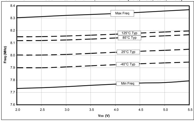
FIGURE 27-38: INTRC vs. VDD ACROSS TEMPERATURE (-40°C TO +125°C)
