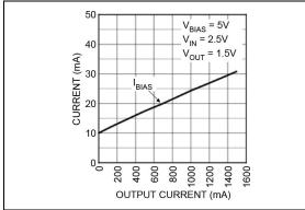
FIGURE 2-13: Bias Current vs. Output Current.
