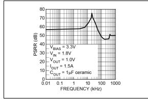
**FIGURE 2-1:** Power Supply Rejection Ratio (Input Supply).
