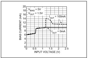
FIGURE 2-18: Bias Current vs. Input Voltage.
