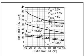
FIGURE 2-12: Bias Current vs. Temperature.
