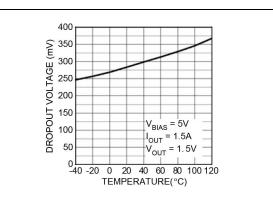
**FIGURE 2-5:** Dropout Voltage vs. Temperature (Input Supply).
