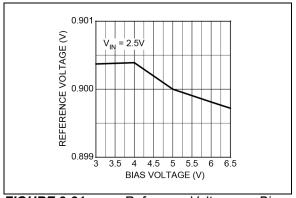
FIGURE 2-21: Reference Voltage vs. Bias Voltage.
