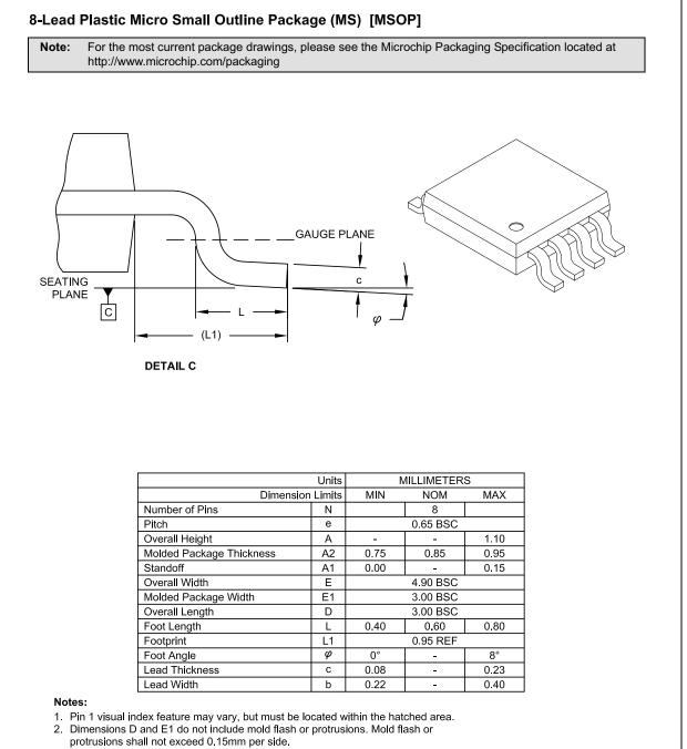
protrusions shall not exceed 0.15mm per side.
