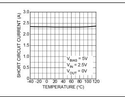
**FIGURE 2-23:** Short-Circuit Current vs. Temperature.
