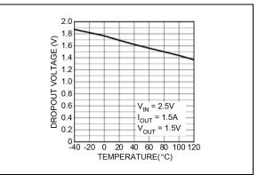
FIGURE 2-6:Dropout Voltage vs.Temperature (Bias Supply).
