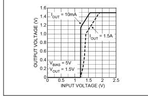
FIGURE 2-7: Dropout Characteristics (Input Voltage).
