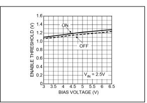
FIGURE 2-24: Enable Threshold vs. Bias Voltage.
