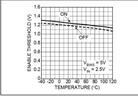
**FIGURE 2-25:** Enable Threshold vs. Temperature.
