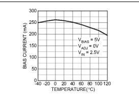
FIGURE 2-11: Maximum Bias Current vs. Temperature.
