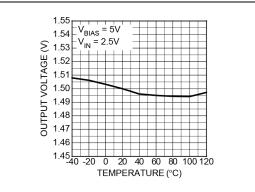
*FIGURE 2-22:* Output Voltage vs. Temperature.
