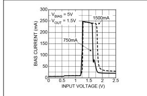
FIGURE 2-19: Bias Current vs. Input Voltage.
