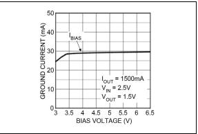
FIGURE 2-17: Bias Current vs. Bias Voltage.
