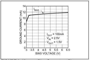
FIGURE 2-15: Bias Current vs. Bias Voltage.
