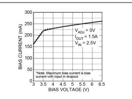
FIGURE 2-10: Maximum Bias Current vs. Bias Voltage.
