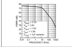
FIGURE 2-2: Power Supply Rejection Ratio (Bias Supply).
