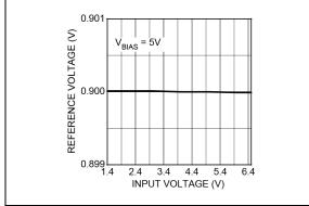
FIGURE 2-20: Reference Voltage vs. Input Voltage.
