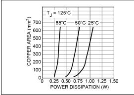
**FIGURE 4-3:** Copper Area vs. Power-MSOP Power Dissipation (T<sub>A</sub>)
