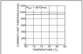
**FIGURE 2-9:** I<sub>LIMIT</sub> vs. Temperature (MIC20X9-0.9A).
