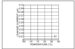
FIGURE 2-15: Switch Leakage Current (MIC20XXA).
