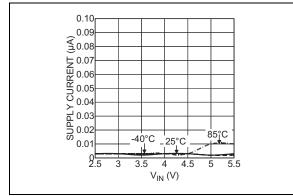
**FIGURE 2-14:** Supply Current Output Disabled (MIC20XXA).
