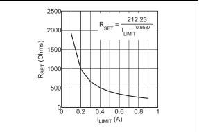
FIGURE 2-18: R<sub>SET</sub> vs I<sub>LIMIT</sub> (MIC20X9A).
