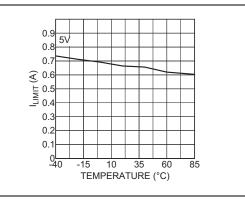
FIGURE 2-16: I<sub>LIMT</sub> vs. Temperature (MIC20X5A).
