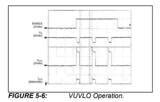
VUVLO and Kickstart operate independently in the MIC2016. If the high current surge allowed by Kickstart causes  $V_{IN}$  to dip below the VUVLO trip point for more than 32 ms, VUVLO will disengage the load, even though the Kickstart timer has not timed out.
