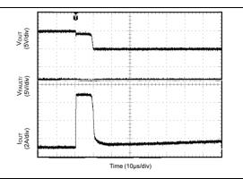
*FIGURE 2-35:* Current Limit Response Time, Stepped Short.
