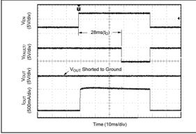
FIGURE 2-31: Enabled Into Short.
