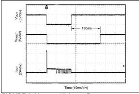
FIGURE 2-39: Kickstart Response Recovery From Thermal Shutdown.
