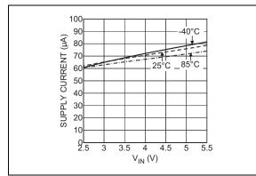
FIGURE 2-13: Supply Current Output Enabled (MIC20XXA).
