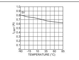
FIGURE 2-4: I<sub>LIMT</sub> vs. Temperature (MIC20XX-0.5).
