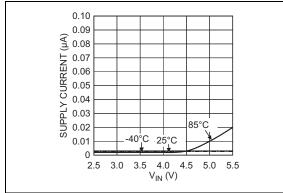
FIGURE 2-2: Supply Current Output Disnabled (MIC20XX).
