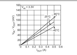
FIGURE 2-23: V<sub>DROP</sub> vs. Temperature (MIC20XXA).
