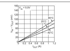
**FIGURE 2-10:** V<sub>DROP</sub> vs. Temperature (MIC20XX-1.2).
