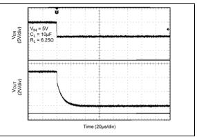
FIGURE 2-29: Enable Turn-Off Delay and Fall Time.
