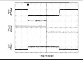
FIGURE 2-32: Current Limit Response, Stepped Short.
