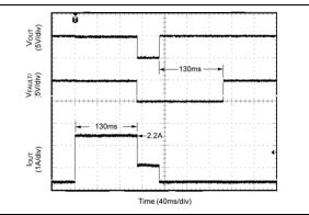
FIGURE 2-41: Kickstart Response 150 ms/2.2A Load Step
