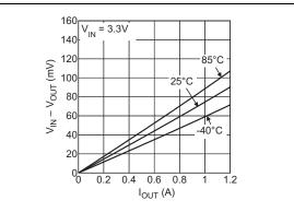
**FIGURE 2-11:** V<sub>DROP</sub> vs. Temperature (MIC20XX-1.2).
