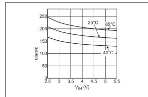
FIGURE 2-19: R<sub>DS(ON)</sub> vs. V<sub>IN</sub> (MIC20XXA).
