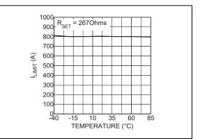
*FIGURE 2-17: I<sub>LIMT</sub> vs. Temperature* (*MIC20X9A-0.8A*).
