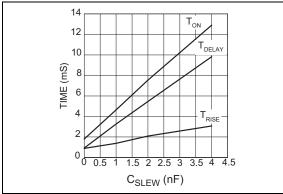
**FIGURE 5-5:** C<sub>SLEW</sub> vs. Turn-On, Delay and Rise Times.
