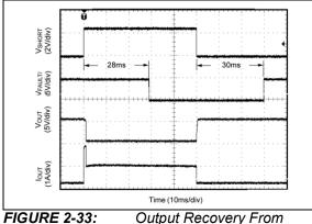
FIGURE 2-33 Short Circuit.
