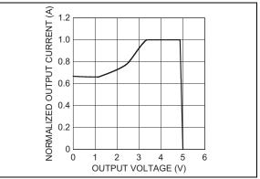
**FIGURE 5-3:** Normalized Output Current vs. Output Voltage (5V).
