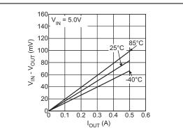
FIGURE 2-22: V<sub>DROP</sub> vs. Temperature (MIC20XXA).
