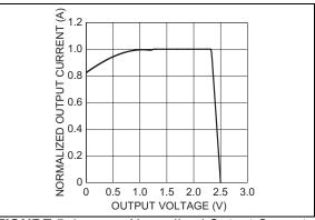
**FIGURE 5-4:** Normalized Output Current vs. Output Voltage (2.5V).
