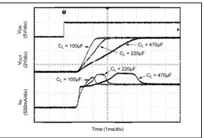
**FIGURE 2-40:** Current Inrush Current Response.
