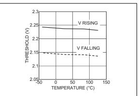
FIGURE 2-24: UVLO Threshold vs. Temperature.
