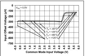
Input Offset Voltage vs. FIGURE 2-5: Common-Mode Input Voltage at  $V_{DD}$  = 5.5V.
