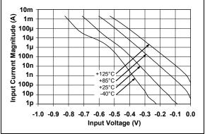
**FIGURE 2-20:** Measured Input Current vs. Input Voltage (below V<sub>SS</sub>).
