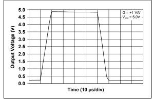
**FIGURE 2-17:** Large-Signal, Noninverting Pulse Response.
