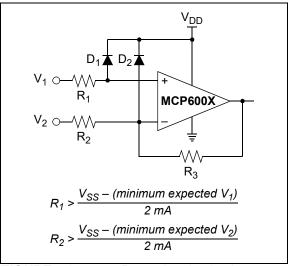
FIGURE 4-2: Protecting the Analog Inputs.
