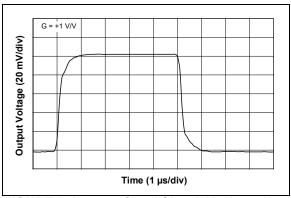
*FIGURE 2-16:* Small-Signal, Noninverting Pulse Response.
