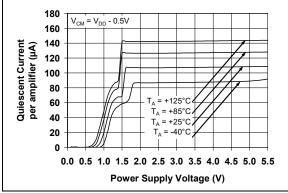
**FIGURE 2-15:** Quiescent Current vs. Power Supply Voltage.
