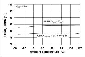
FIGURE 2-9: CMRR, PSRR vs. Ambient Temperature.
