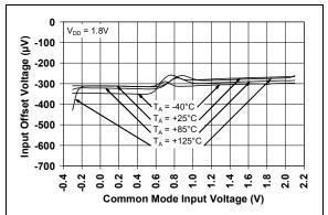
Input Offset Voltage vs. FIGURE 2-4: Common-Mode Input Voltage at  $V_{DD}$  = 1.8V.
