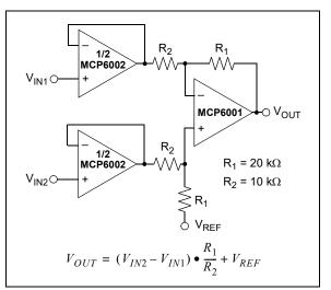
**FIGURE 4-7:** Instrumentation Amplifier with Unity Gain Buffer Inputs.
