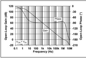
FIGURE 2-11: Open-Loop Gain, Phase vs. Frequency.
