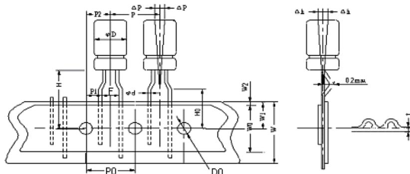
Size F means the distance after forming between the centers of the two lead pins.
