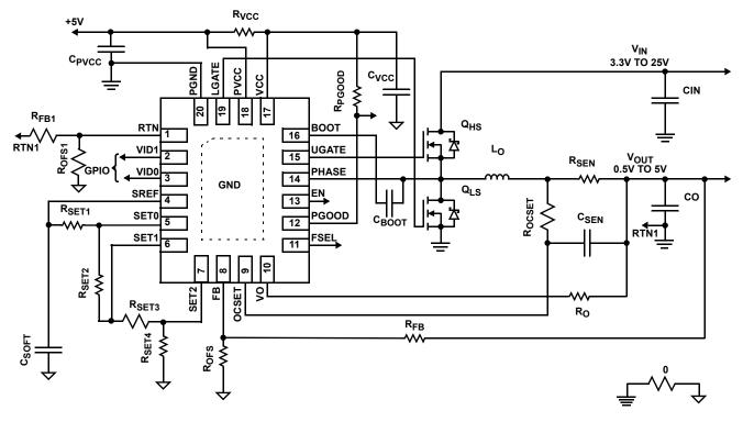
FIGURE 7. ISL95870B APPLICATION SCHEMATIC WITH FOUR OUTPUT VOLTAGE SETPOINTS AND RESISTOR CURRENT SENSE
