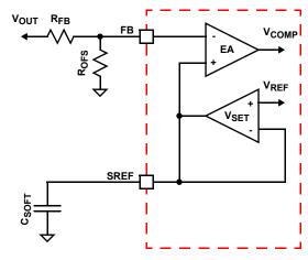
FIGURE 9. ISL95870 VOLTAGE PROGRAMMING CIRCUIT
