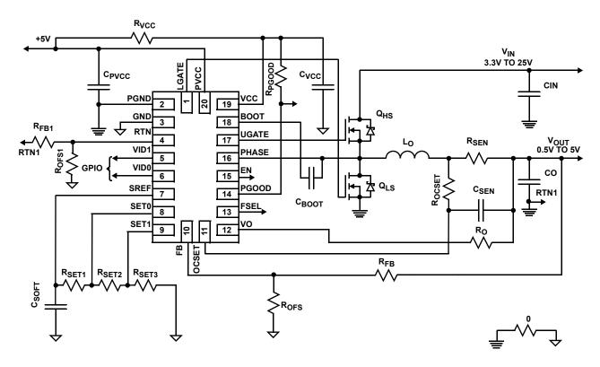
FIGURE 5. ISL95870A APPLICATION SCHEMATIC WITH FOUR OUTPUT VOLTAGE SETPOINTS AND RESISTOR CURRENT SENSE
