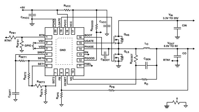
FIGURE 6. ISL95870B APPLICATION SCHEMATIC WITH FOUR OUTPUT VOLTAGE SETPOINTS AND DCR CURRENT SENSE
