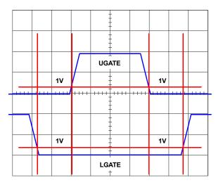
FIGURE 18. GATE DRIVE ADAPTIVE SHOOT-THROUGH PROTECTION
