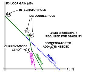
FIGURE 13. UNCOMPENSATED INTEGRATOR OPEN-LOOP RESPONSE
