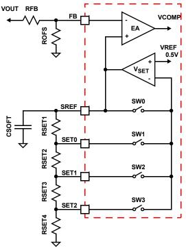
FIGURE 11. ISL95870B VOLTAGE PROGRAMMING CIRCUIT
