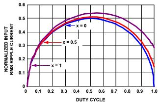
FIGURE 19. NORMALIZED INPUT RMS CURRENT FOR EFF = 1
