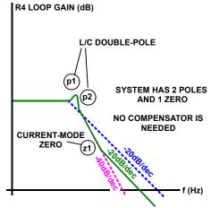
FIGURE 15. UNCOMPENSATED R4 OPEN-LOOP RESPONSE
