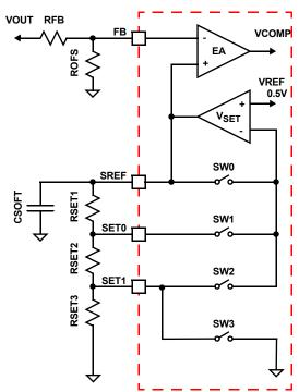
FIGURE 10. ISL95870A VOLTAGE PROGRAMMING CIRCUIT
