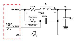
FIGURE 17. OVERCURRENT PROGRAMMING CIRCUIT
