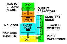
FIGURE 29. TYPICAL POWER COMPONENT PLACEMENT
