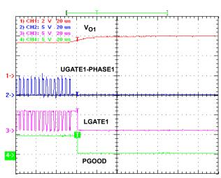
FIGURE 22. TRI-STATE OVERVOLTAGE PROTECTION,  $V_{IN}$  = 12V,  $V_{O}$  = 3.3V, NO LOAD
