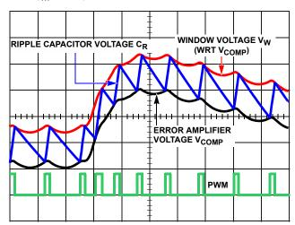
FIGURE 23. MODULATOR WAVEFORMS DURING LOAD TRANSIENT
