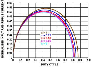
FIGURE 28. NORMALIZED RMS INPUT CURRENT
