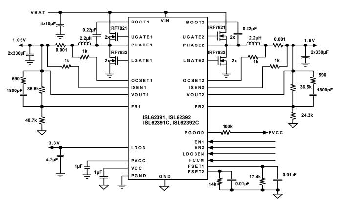
FIGURE 4. TYPICAL CHIP SET APPLICATION CIRCUIT WITH RESISTOR SENSE
