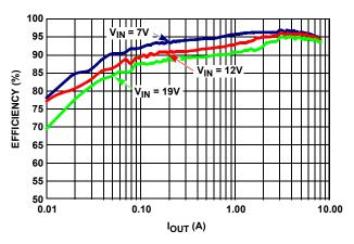
FIGURE 6. CHANNEL 2 EFFICIENCY AT  $V_O$  = 5V, DEM OPERATION. HIGH-SIDE 1xIRF7821,  $r_{DS(ON)}$  = 9.1m $\Omega$ ; LOW-SIDE 1xIRF7832,  $r_{DS(ON)}$  = 4m $\Omega$ ; L = 4.7 $\mu$ H, DCR = 14.3m $\Omega$ ; CCM  $F_{SW}$  = 330kHz
