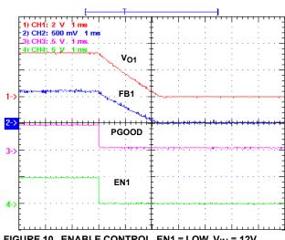
FIGURE 10. ENABLE CONTROL, EN1 = LOW,  $V_{IN}$  = 12V,  $V_{O}$  = 3.3V,  $I_{O}$  = 5A
