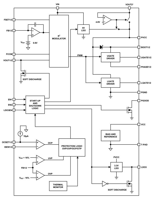
\*In addition to being used for regulation, VOUT2 will also provide power for PVCC when it is programmed to 5V.
