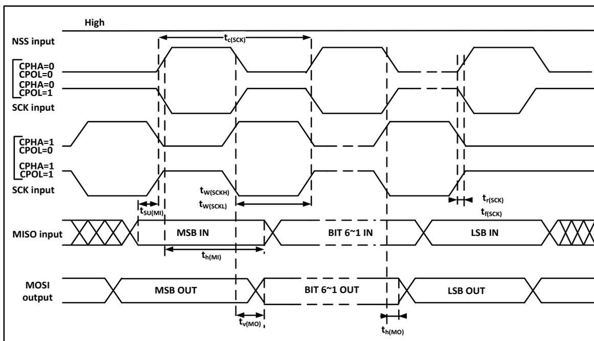
Note: The measuring points are set at CMOS levels:  $0.3V_{DD}$  and  $0.7V_{DD}$ .
