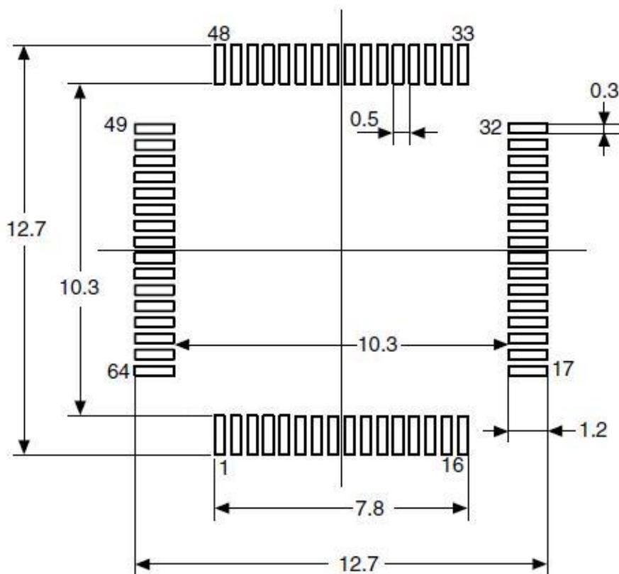
Figure 26 LQFP64-64 pins, 10×10mm package identification
