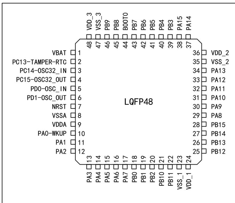
图 5 Distribution Diagram of APM32E103xCxE Series QFN48 Pins
