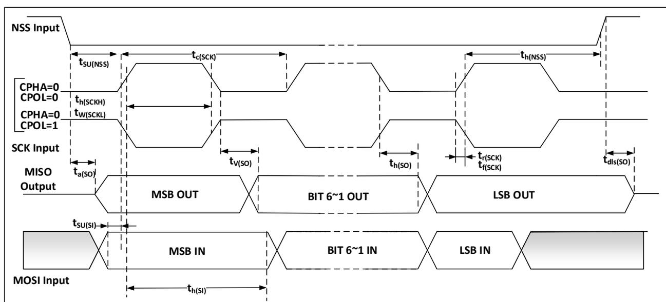
Figure 16 SPI Timing Diagram - Slave Mode and CPHA=1
