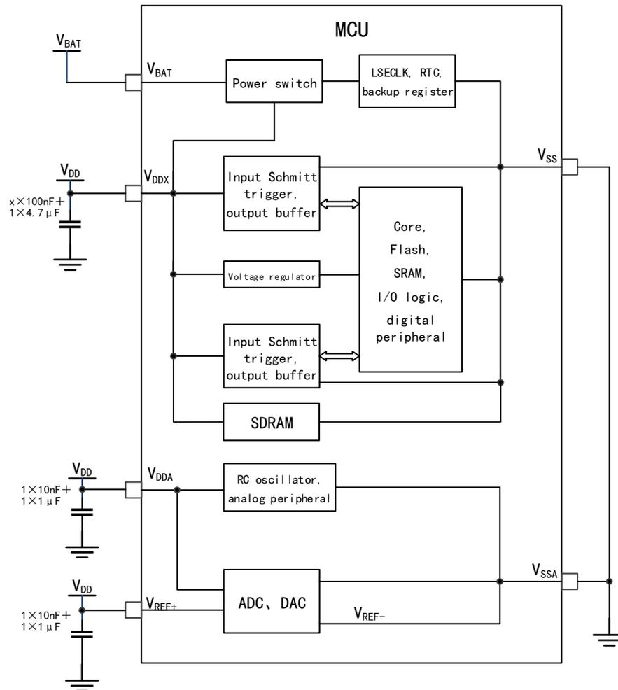
Notes:  $V_{DDX}$  in the figure means the number of  $V_{DD}$  is  $x$
