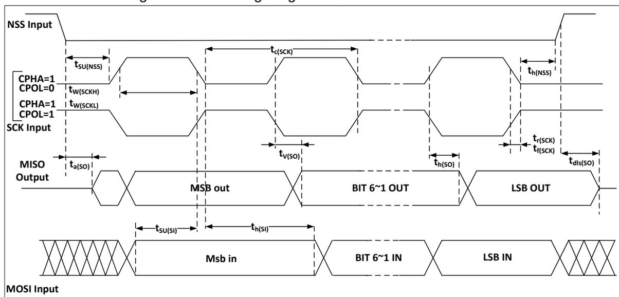
Note: The measuring points are set at CMOS levels:  $0.3V_{DD}$  and  $0.7V_{DD}$ .
