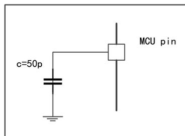
Figure 11 Pin Input Voltage Measurement Scheme
