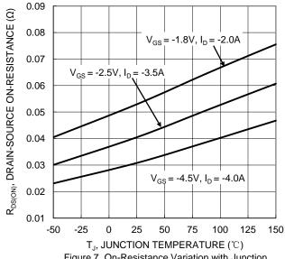
Figure 7. On-Resistance Variation with Junction Temperature
