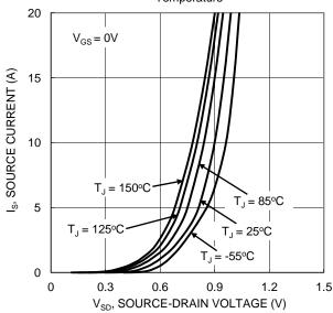
Figure 9. Diode Forward Voltage vs. Current
