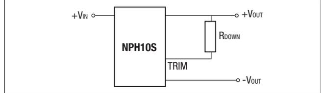
When the output voltage is trimmed up, output current must be derated so that the maximum output power 10W is not exceeded.
