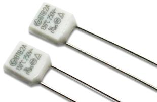
The following product specifications apply to fuses of the BTB series. The BTB series consists of thermal cutoff fuses for over-temperature protection. The BTB series thermal fuses are widely used in various applications such as transformers, adapters, secondary batteries, household appliances, gas water heaters, lighting and other heating equipment.
