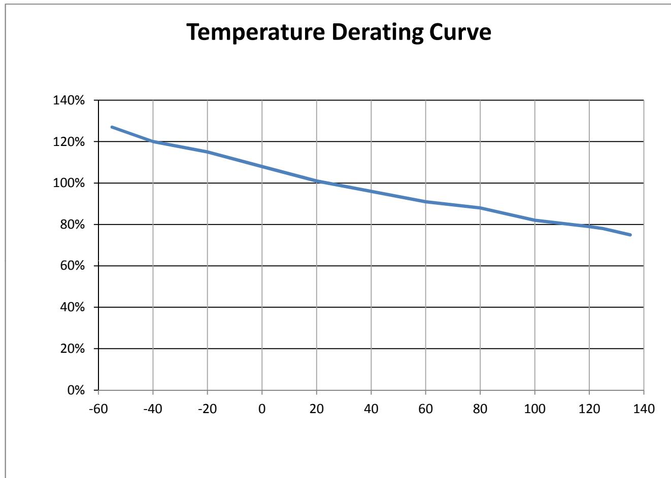
$$\text{Calculation for ideal fuse selection} = \frac{\text{Operating Current(A)}}{\text{Rating } (\% \times 0.75)}$$
