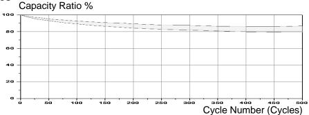
Note: The curve is based on the test result of 20 pcs of batteries
