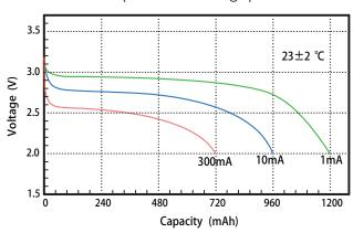
2. Typical discharge profiles with different current (at discharge stable phase)
