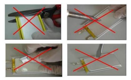
Top Sealing Edge: Sealing edge on the top of the Cell is very flimsy and easy to be delaminated. Do not bend or fold this area.
