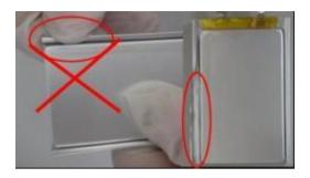
Mechanical Shock:Do not drop shock or bend Cell body
