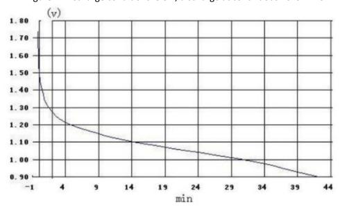
Figure 2. Discharge conditions: 75 $\Omega$ , discharge at 20°C ± 2°C, discharge for 4 hours per day.
