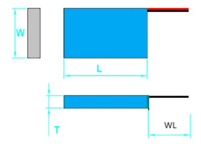
L: ≤61.0mm W: ≤38.0mm T: ≤10.5mm WL: 150mm Connector: NA Marking: 503759 3.7V 2400mAh 8.88Wh +YYMMDD
