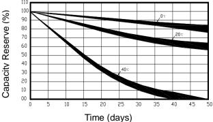
The specification is suitable for the performance of NI-MH rechargeable battery produced
