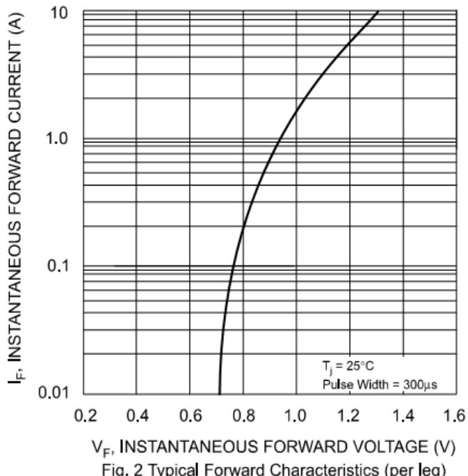
Fig. 2 Typical Forward Characteristics (per leg)
