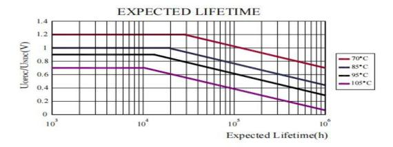
The temperatures-curves are the case-temperatures measured at the hottest point of the capacitor has reached its thermal equilibrium.
