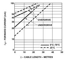
Figure 3. Guaranteed System Performance with Standard Cable (HFBR-15X1/25X1).
