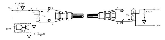
Figure 2. Typical 5 MBd Interface Circuit.
