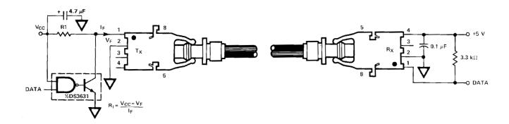
Figure 20. Typical 40 kBd Interface Circuit.
