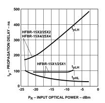
Figure 8. Typical Link Propagation Delay vs. Optical Power.
