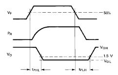
Figure 6. Propagation Delay Test Waveforms.
