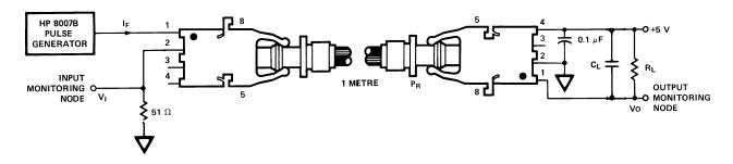
Figure 23. 40 kBd Propagation Delay Test Circuit.
