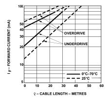
Figure 4. Guaranteed System Performance with Improved Cable (HFBR-15X1/25X1).
