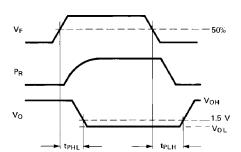
Figure 26. Propagation Delay Test Waveforms.
