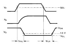
Figure 19. Propagation Delay Test Waveforms.
