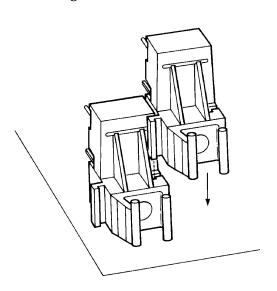
Figure 1. Interlocked (Stacked) Horizontal or Vertical Packages.
