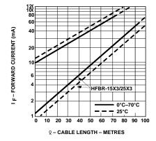
Figure 21. Guaranteed System Performance with Standard Cable.
