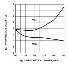
Figure 25. Typical Link Propagation Delay vs. Optical Power.
