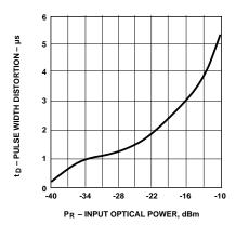
$\begin{array}{ll} \textbf{Figure 24. Typical Link Pulse Width Distortion vs.} \\ \textbf{Optical Power.} \end{array}$
