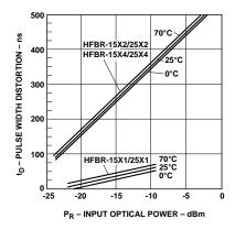
$\label{eq:continuous} \textbf{Figure 7. Typical Link Pulse Width Distortion vs.} \\ \textbf{Optical Power.}$
