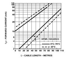
Figure 22. Guaranteed System Performance with Improved Cable.
