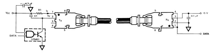
Figure 11. Required 1 MBd Interface Circuit.
