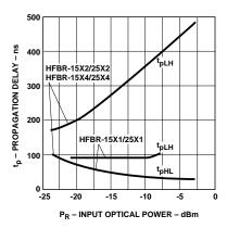
Figure 17. Pulse Width Distortion vs. Optical Power.
