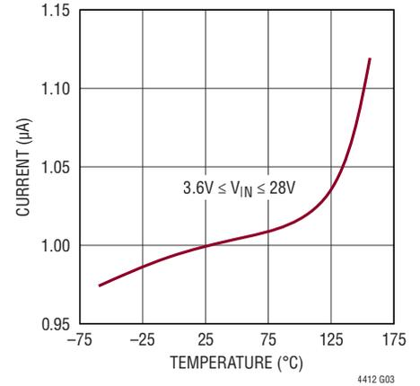
**I<sub>LEAK</sub> vs Temperature**
