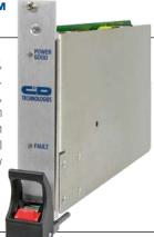
DC/DC A family of high reliability, 200W Watt power supplies for 3U CompactPCI™ systems. These hot-swap, N+1 redundant supplies are just 4HP (1 card slot) wide making them the narrowest in the industry. Standard features include 47-pin I/O connector, active current sharing and no load operation. Models are also available with an IPMI option.
