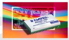
The ADCDS family are application-specific video signal processors designed for electronic-imaging applications that employ CCDs (Charge Coupled Devices) as their photodetector.
